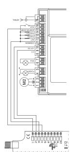
Example connection with Nice MC 424 controller (Note! COMMON has a positive potential)
